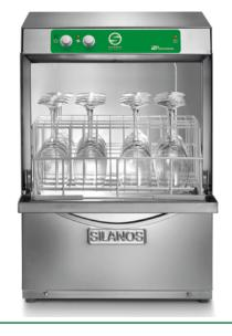
Control panel Electromechanical Body Single-skinned Rinse arm Technopolymer Wash arms Stainless steel External dimensions **465x510x645** mm Depth with open door 810 mm Usable wash height **255** mm **270** mm Door height Rack dimensions 400x400 mm Wash tank volume **12** lt Water usage 2.4 lt/cycle Wash pump 0.17 kW **1.6** kW Tank element Boiler element 2.8 kW Total installed power 2.97 kW **120** sec Cycles Hourly production **30** rack/h **230** V**/50** Hz Voltage Noise level **48** dBA
