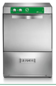
Control panel Electromechanical Body Single-skinned Rinse arm Technopolymer Wash arms Stainless steel External dimensions **415x465x595** mm Depth with open door **710** mm Usable wash height **205** mm Door height **220** mm Rack dimensions 350x350 mm Wash tank volume **11** lt Water usage 2.4 lt/cycle Wash pump 0.17 kW **1.6** kW Tank element Boiler element 2.6 kW Total installed power 2.77 kW **120** sec Cycles Hourly production **30** rack/h **230** V**/50** Hz Voltage Noise level **48** dBA
